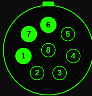
8-PIN CASE CONNECTOR — VIEWED FROM TRANS SIDE
